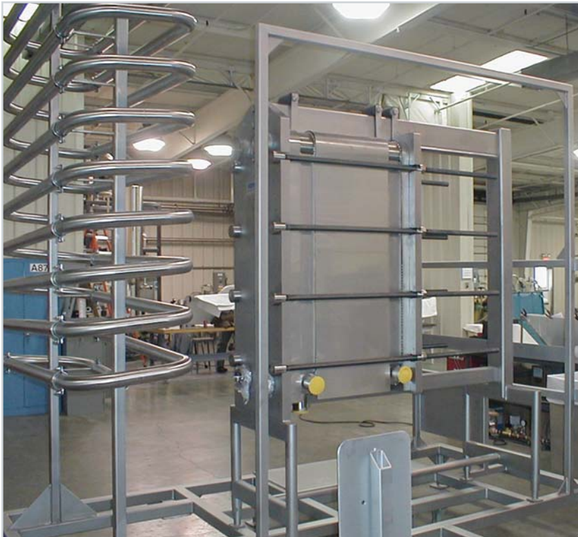
A mixing skid, complete with a stainless steel Accu-Therm, used for processing liquor.
